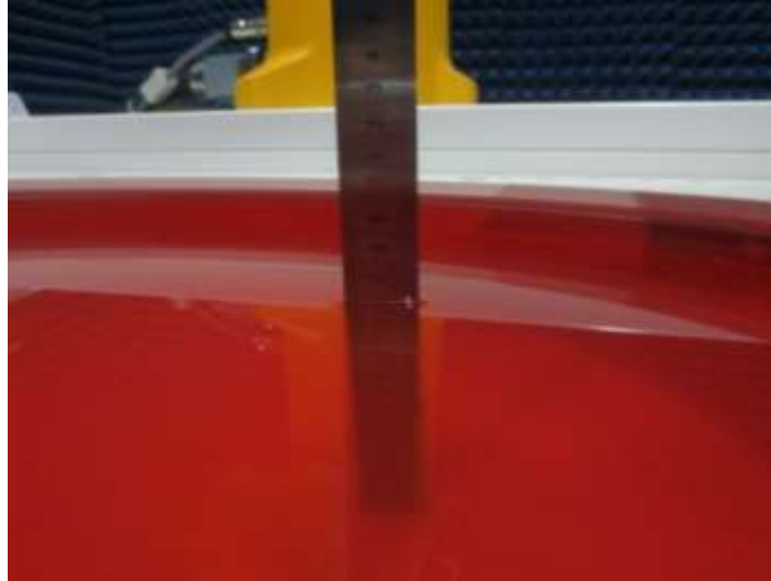
Fig. 9.1 Photo of Liquid Height for Body SAR of Twin Phantom (2000MHz~2600MHz) (depth>15cm)
