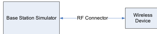
Figure 9-4 Power Measurement Setup – NR FDD
