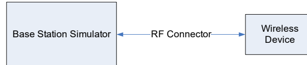
Figure 9-3 Power Measurement Setup
