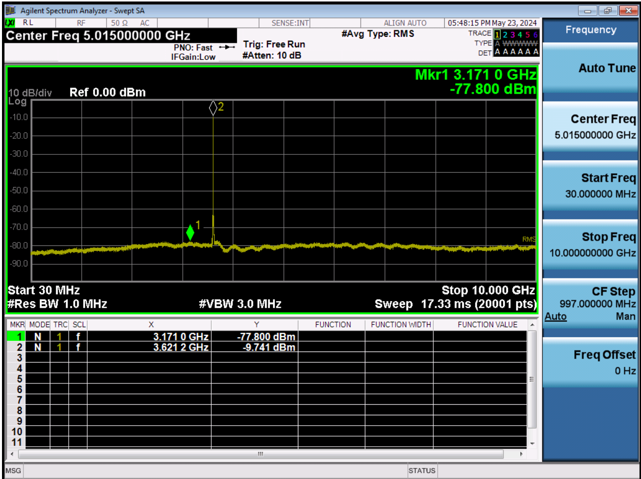
BAND 48. Conducted Spurious Plot 1 (10 MHz Ch.55990 QPSK RB 1, Offset 0)
