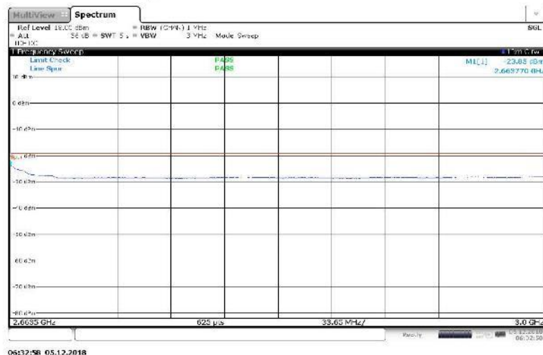
Figure 60 Spurious Emissions (2.6635 GHz – 3 GHz) – 16QAM (2655 MHz, 15 MHz Channel BW)
