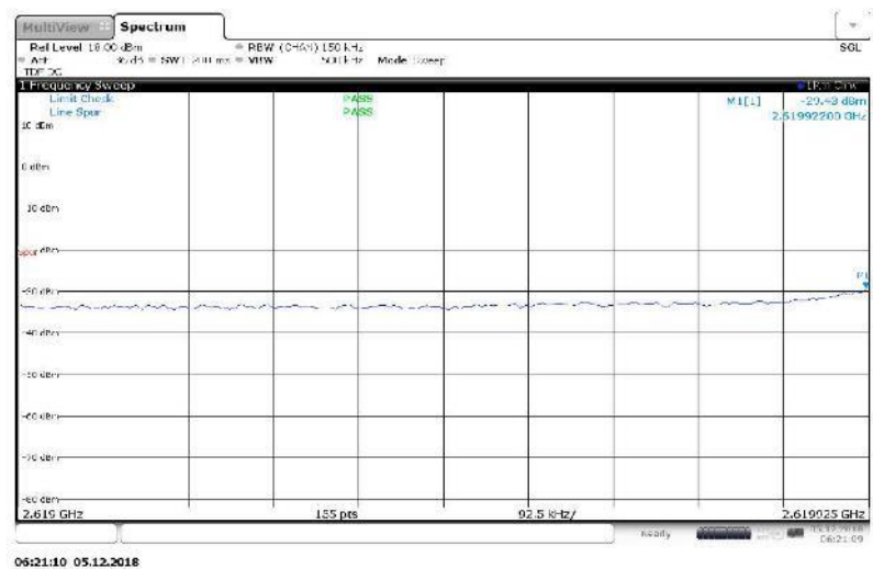
Figure 63 Spurious Emissions (Lower Band Edge) – 64QAM (2627.5 MHz, 15 MHz Channel BW)
