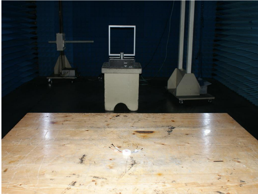
Photograph 1: Set-up for Radiated Spurious Emission, 9KHz - 30MHz
