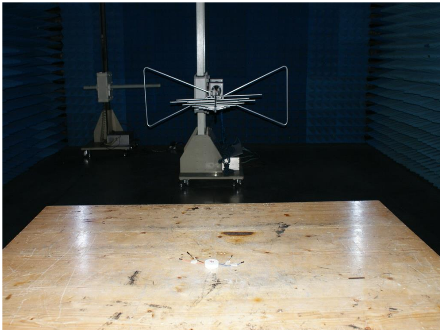
Photograph 2: Set-up for Radiated Spurious Emission, 30MHz - 1GHz
