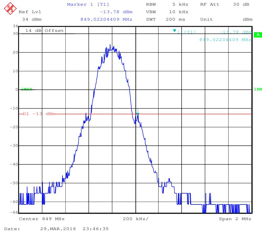
**PCS Band, Left Band Edge for GSM (GMSK) Mode**
