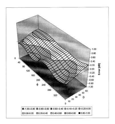
Spherical Isotropy Error < ± 0.4 dB
