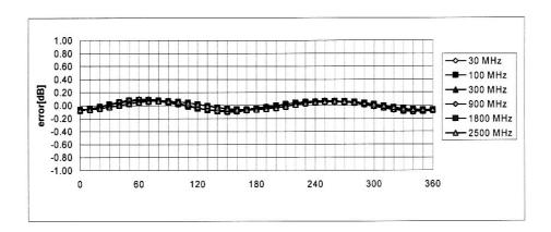
Axial Isotropy Error < ± 0.2 dB
