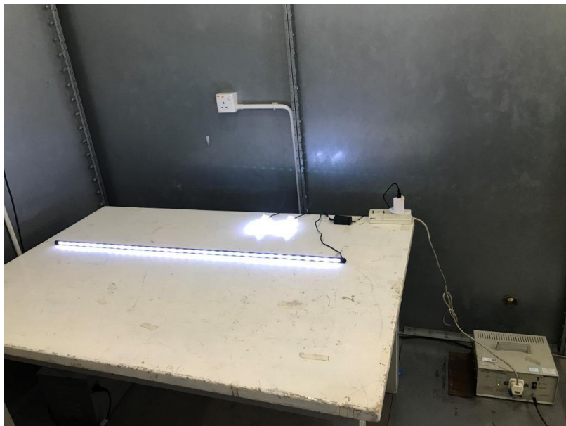
Measurement of Conducted Emission Test Set Up
