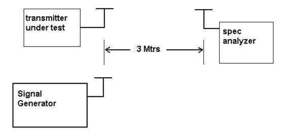
METHOD OF MEASUREMENT: The procedure used was TIA/EIA STANDARD 603. The spectrum was scanned from 30 to at least the tenth harmonic of the fundamental using a HP model 8566B spectrum analyzer and an appropriate antenna. Measurements were made at the open field test site of TIMCO ENGINEERING INC. located at 849 NW SR 45 Newberry, Florida 32669.
