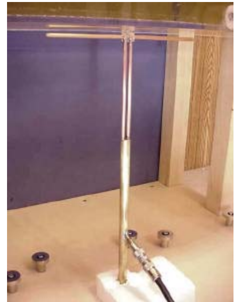
450MHz System Check Setup Photograph
