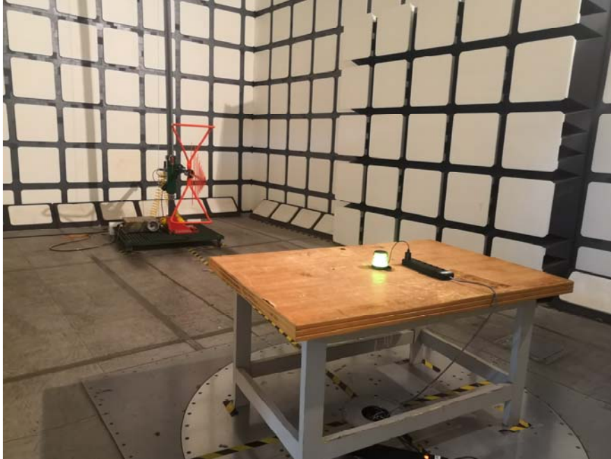
Radiated Emissions View (Below 1 GHz)
