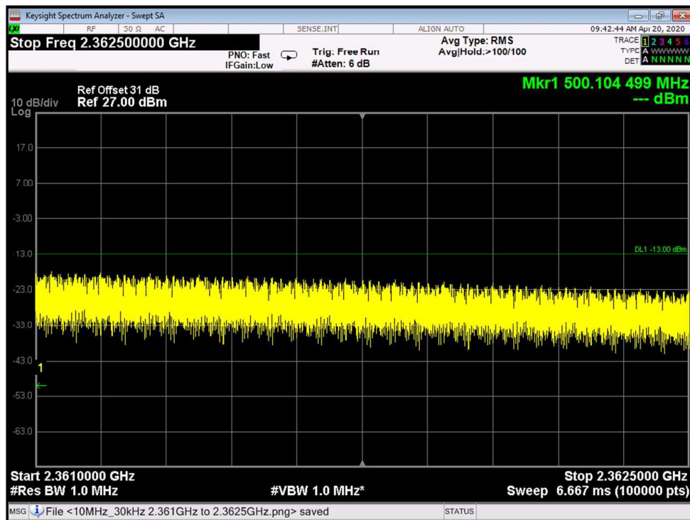
Figure 104: Spurious Emissions at Antenna Terminal 256QAM, 2355.0MHz, B.W. 10MHz, Sub Carrier 60kHz
