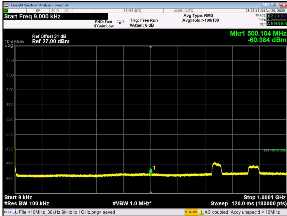
Figure 101: Spurious Emissions at Antenna Terminal 256QAM, 2355.0MHz, B.W. 10MHz, Sub Carrier 60kHz
