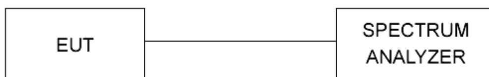
Figure 1 - Bandwidth Measurements Test Setup
