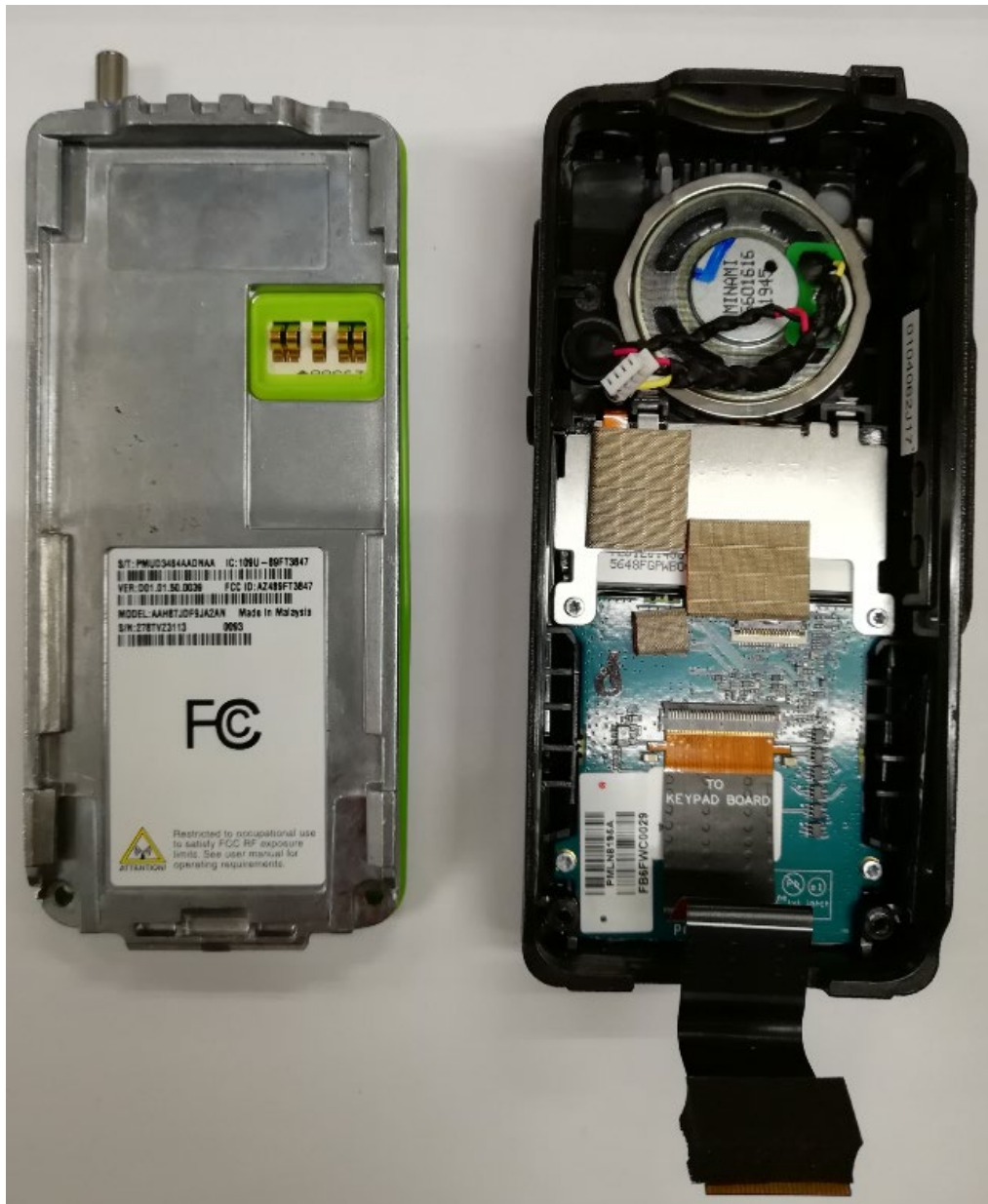
Chassis and Housing (Back side) -Full Keypad (FKP) model, AAH87JDF9JA2AN-
