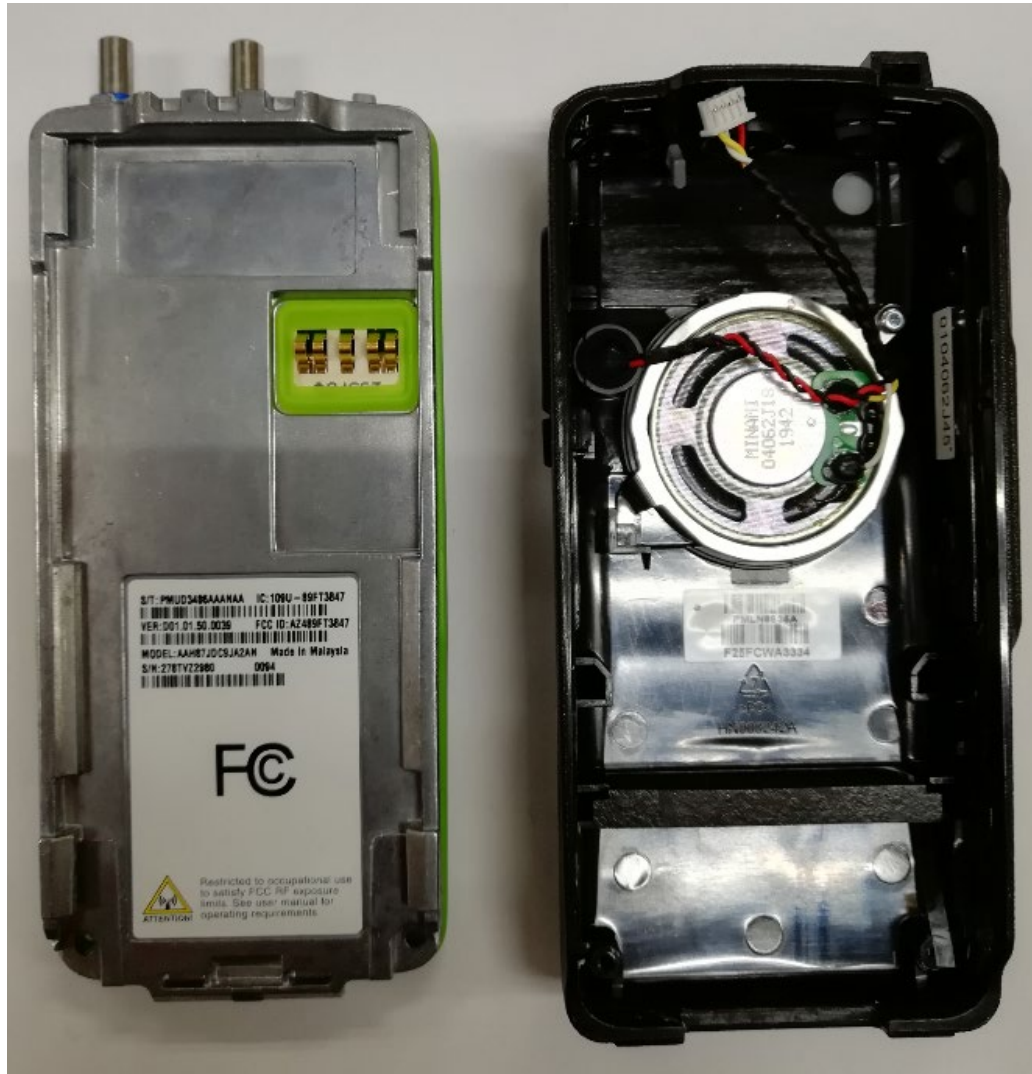
Chassis and Housing (Back side) -Non Keypad (NKP) model, AAH87JDC9JA2AN-
