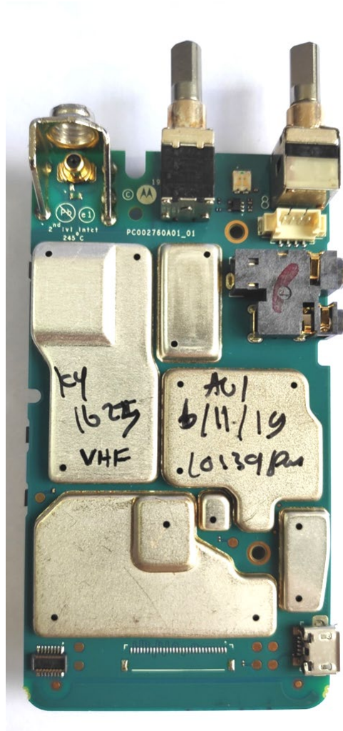
RF board with Shields (Top) -Non Keypad (NKP) model, AAH87JDC9JA2AN-
