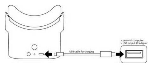
Charge the battery by connecting the USB terminal of the PC or a commercially available USB output AC adapter to the charging terminal of the main unit with the supplied USB charging cable.
