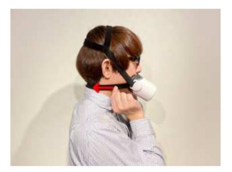
**6. Adjust the buckle position.** Adjust the headband so that the buckle is centered behind the neck.
