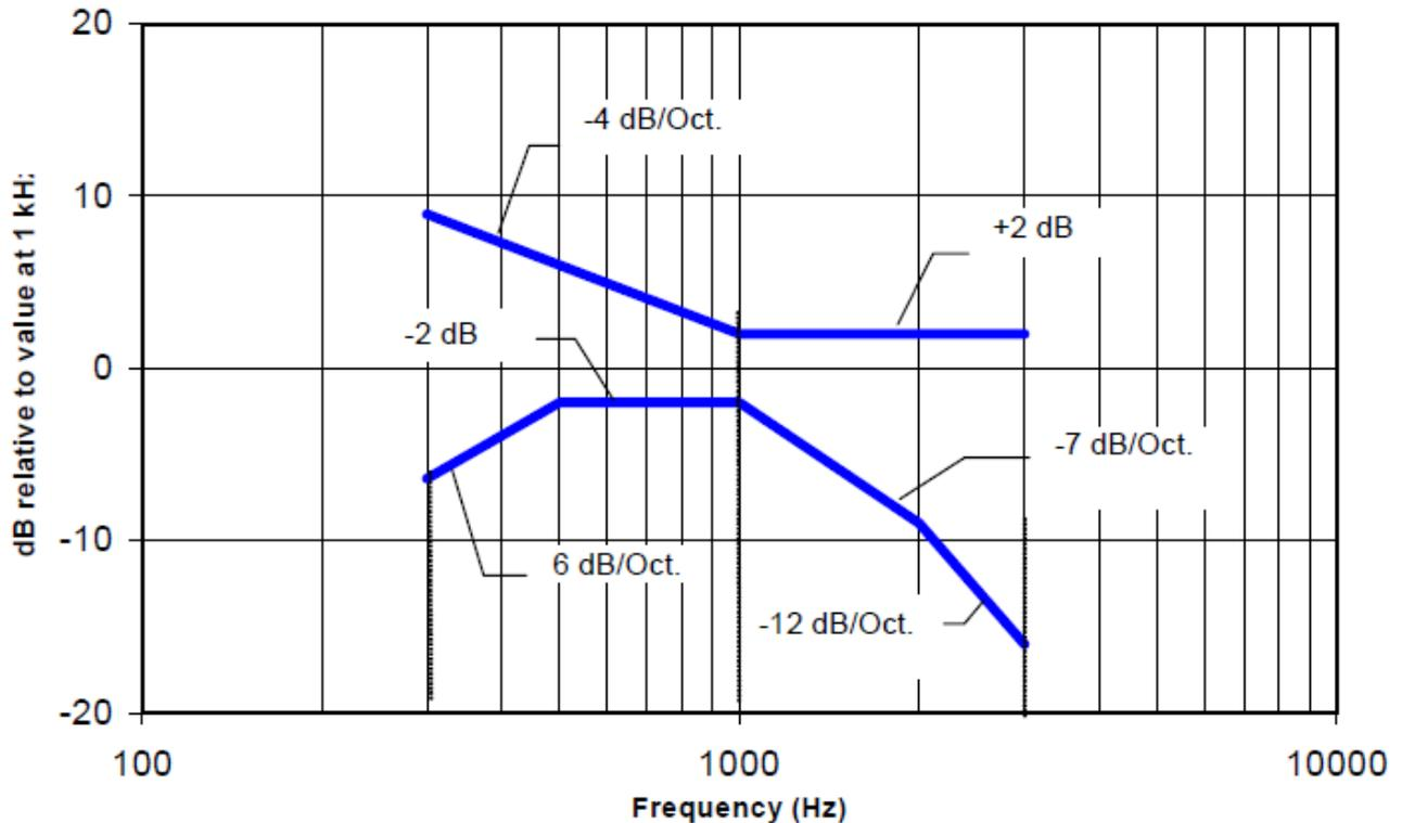
Figure 2 —Magnetic field frequency response for WDs with a field that exceeds  $-15\text{dB(A/m)}$  at 1 kHz
