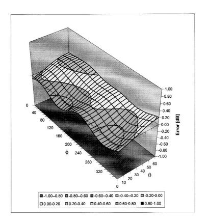
Spherical Isotropy Error < ± 0.4 dB
