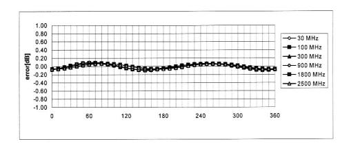
Axial Isotropy Error < ± 0.2 dB
