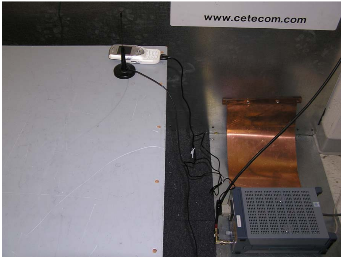
Test setup – AC Line Conducted Emissions
