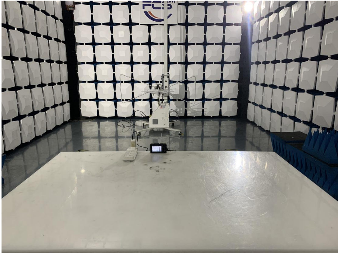
Above 1GHz for radiated emission test setup
