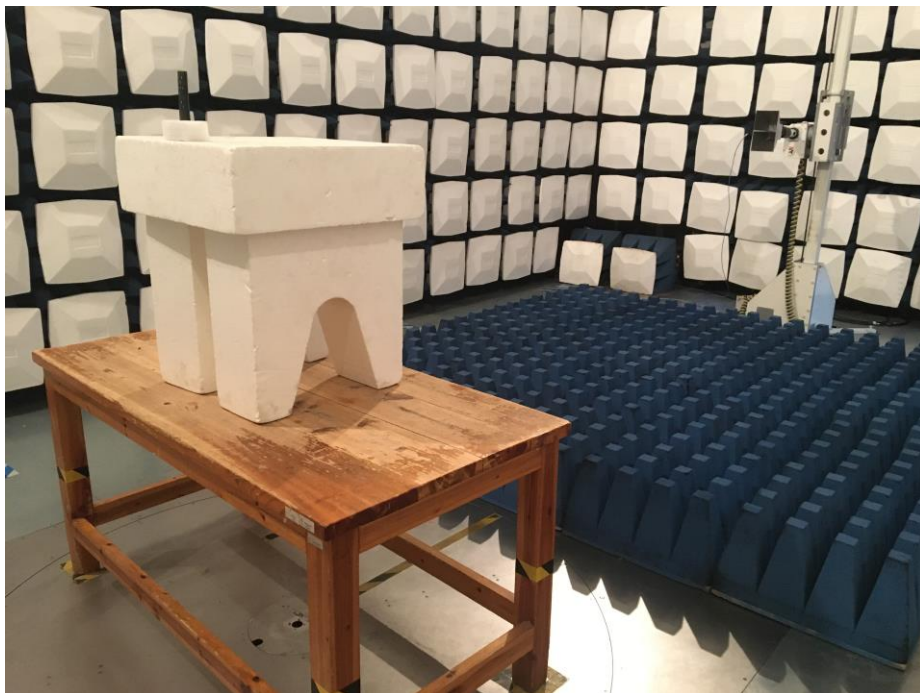
Test Setup For Radiated Emission (Above 1GHz)
