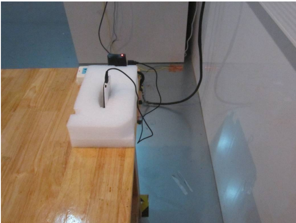
Conducted Emissions Test Setup Side View
