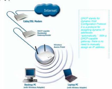
**Requirements:** A Residential Gateway/Router connected with an Ethernet (CAT5) cable to an 802.11g Access Point.
