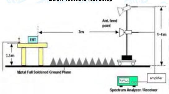
**Above 1GHz Test Setup**
