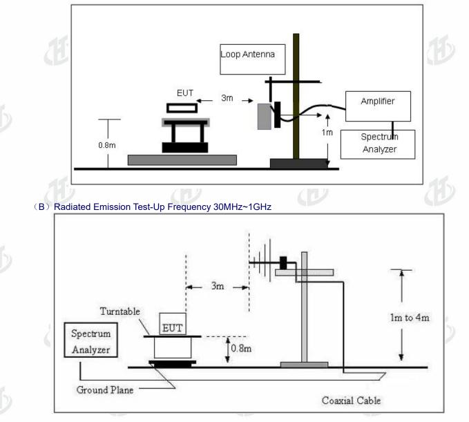
The radiated emission test were performed in the 3 meters chamber test site, using the setup accordance with the ANSI C63.10-2013. The specification used was the FCC 15.209 and FCC 15.205 limit.
