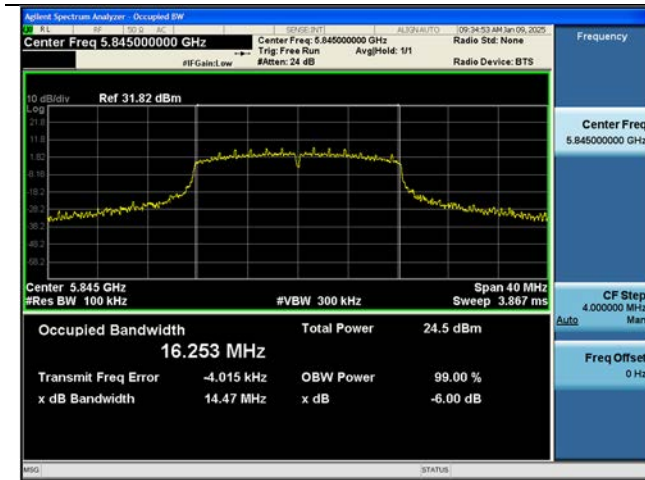
802.11ac(VHT20) 6 dB Bandwidth (CH 149)
