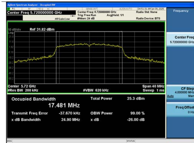
802.11ac(VHT40) 26 dB Bandwidth (CH 142)
