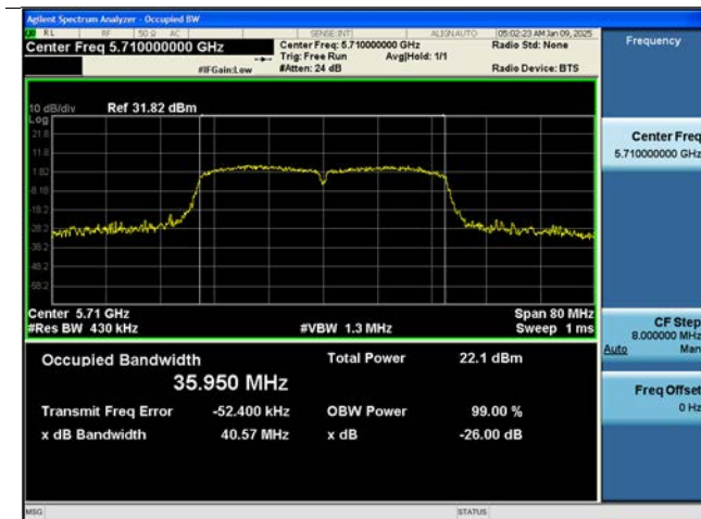
802.11ac(VHT40) 26 dB Bandwidth (CH 142)
