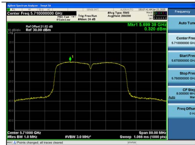
802.11ac(VHT40) UNII 2C Band
