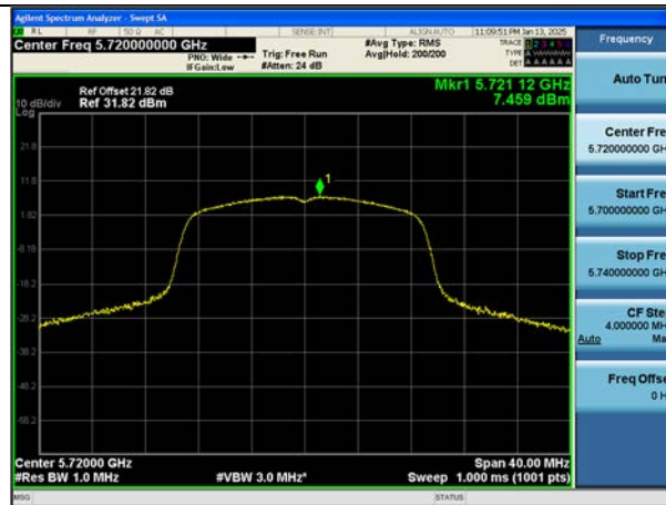
Bandwidth 40M, 802.11ac(VHT40) (Ch. 142)
