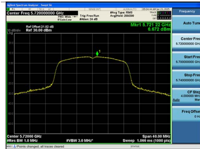
802.11ac(VHT20) UNII 2C Band
