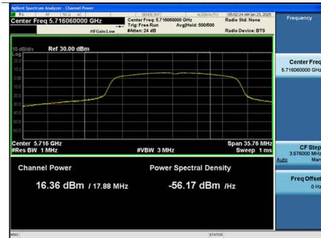
802.11ac(VHT20) UNII 2C Band
