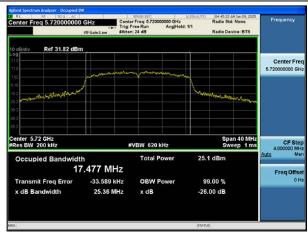
802.11n(HT40) 26 dB Bandwidth (CH 102)
