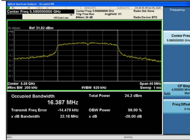
802.11ac(VHT20) 26 dB Bandwidth (CH 144)
