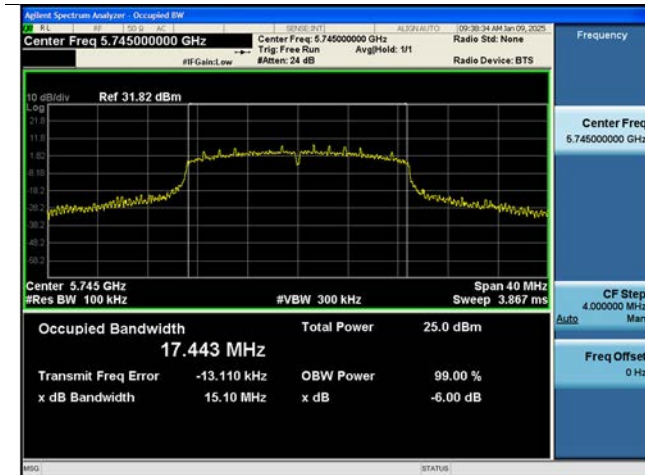
802.11ac(VHT40) 6 dB Bandwidth (CH 159)
