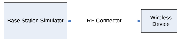
Figure 10-4 Power Measurement Setup – NR FDD
