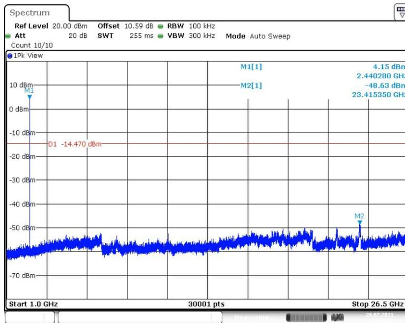
Fig.22 Conducted Spurious Emission (CH19, 1GHz-26.5GHz), LE 1M
