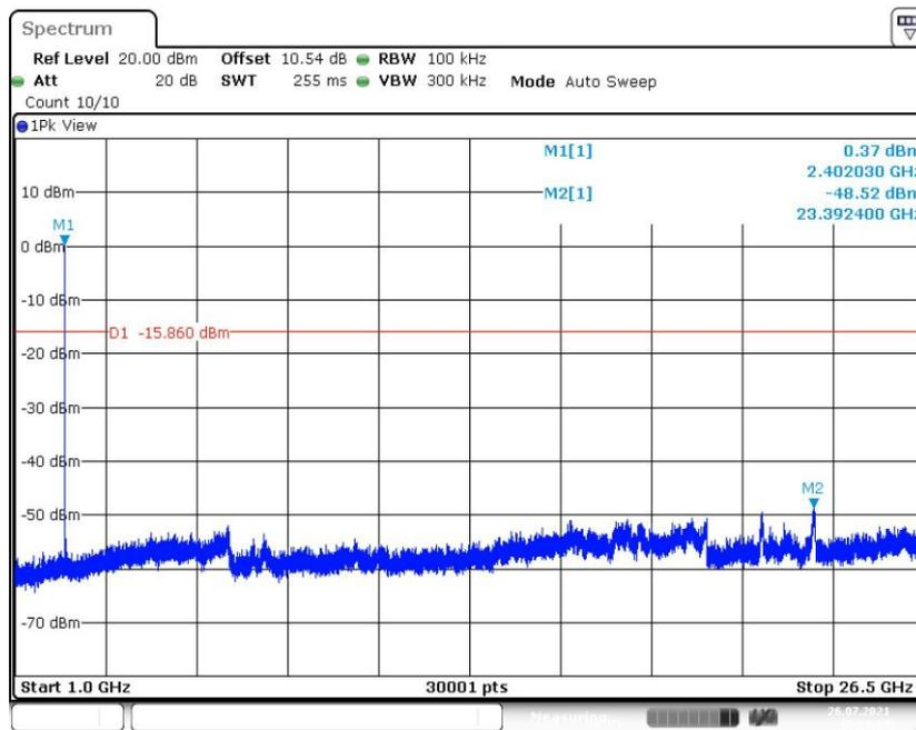
Fig.28 Conducted Spurious Emission (CH0, 1GHz-26.5GHz), LE 2M
