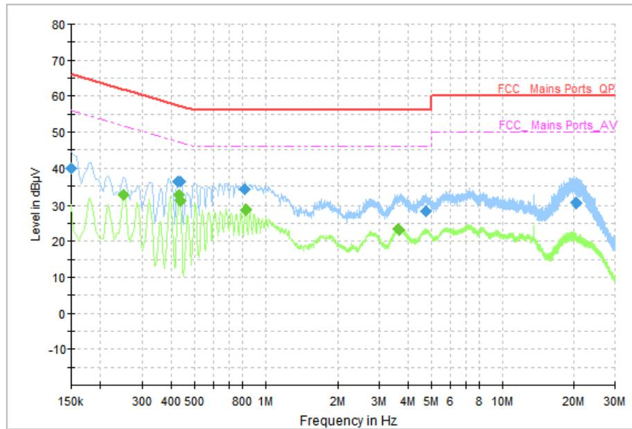
Fig.54 AC Power line Conducted Emission (Idle), LE 2M
