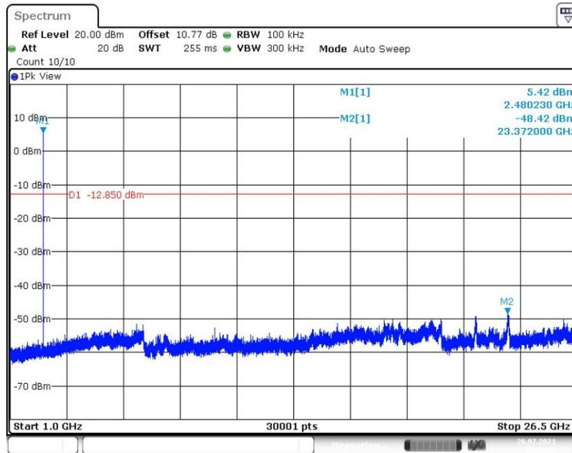
Fig.25 Conducted Spurious Emission (CH39, 1GHz-26.5GHz), LE 1M
