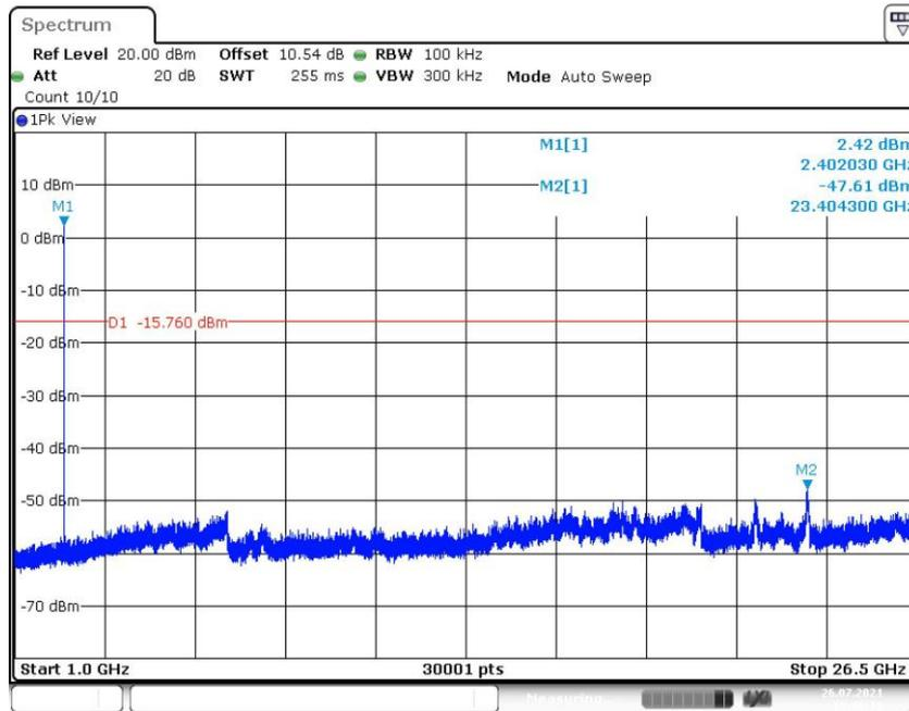
Fig.19 Conducted Spurious Emission (CH0, 1GHz-26.5GHz), LE 1M
