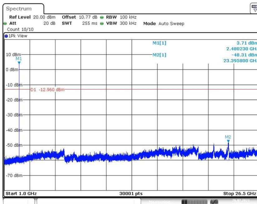
Fig.34 Conducted Spurious Emission (CH39, 1GHz-26.5GHz), LE 2M
