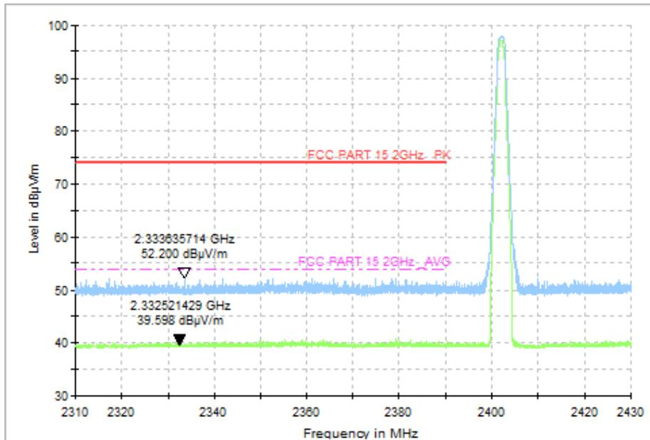
Fig.38 Radiated Band Edges (CH0, 2380GHz~2450GHz), LE 1M
