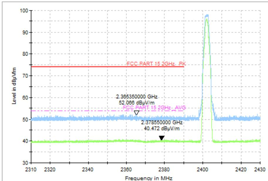
Fig.46 Radiated Band Edges (CH0, 2380GHz~2450GHz), LE 2M
