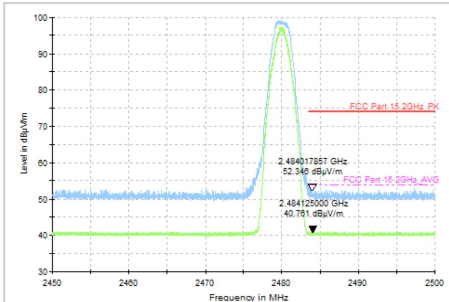
Fig.47 Radiated Band Edges (CH39, 2450GHz~2500GHz), LE 2M
