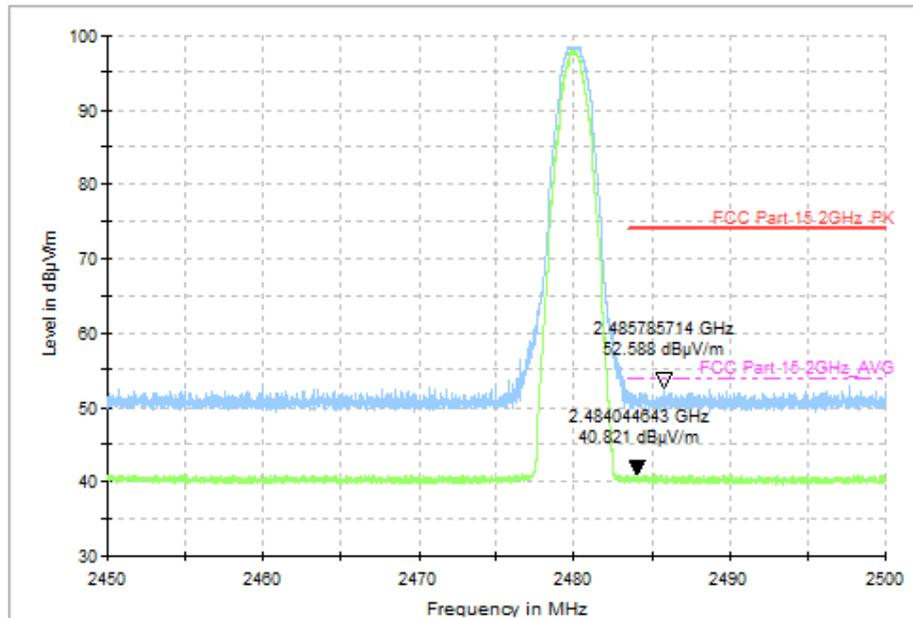
Fig.39 Radiated Band Edges (CH39, 2450GHz~2500GHz), LE 1M
