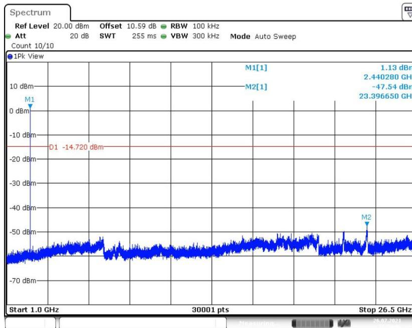
**Fig.31 Conducted Spurious Emission (CH19, 1GHz-26.5GHz), LE 2M**
