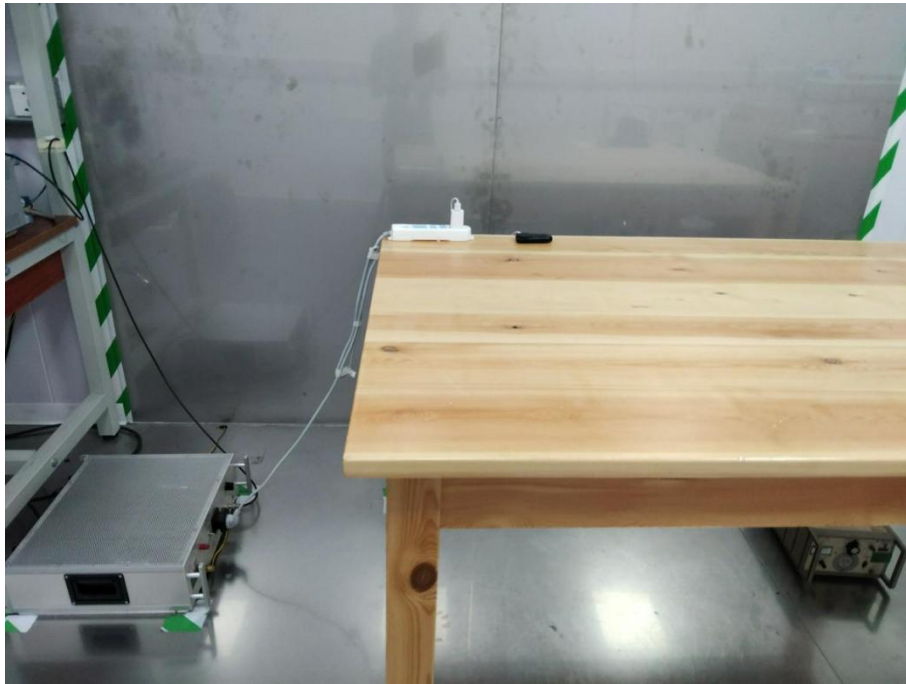
Conducted Emission at AC power line
