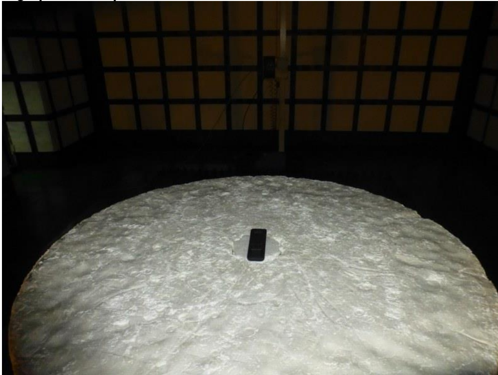
Photograph 3: Set-up for Radiated Emission of 1 – 5GHz for IC
