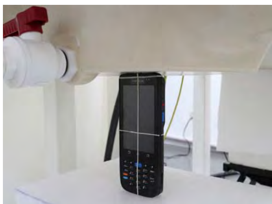
Fig.11 EUT Top side to flat phantom
