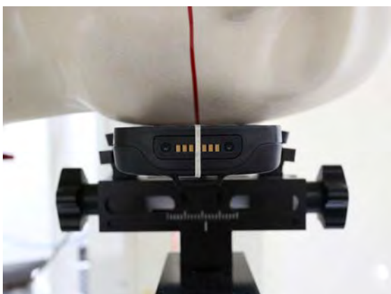
Fig.5 Left Head Section / Cheek-Touch Position
