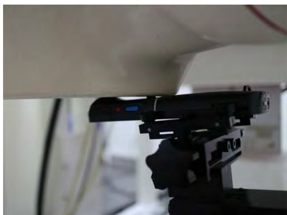
Fig.10 EUT Back side to flat phantom
