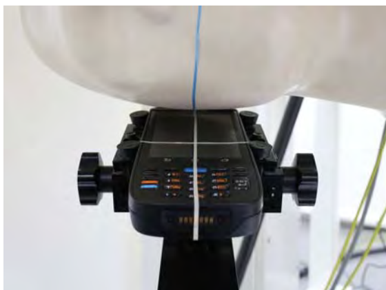
Fig.4 Right Head Section / Ear-Tilt Position(15°)
