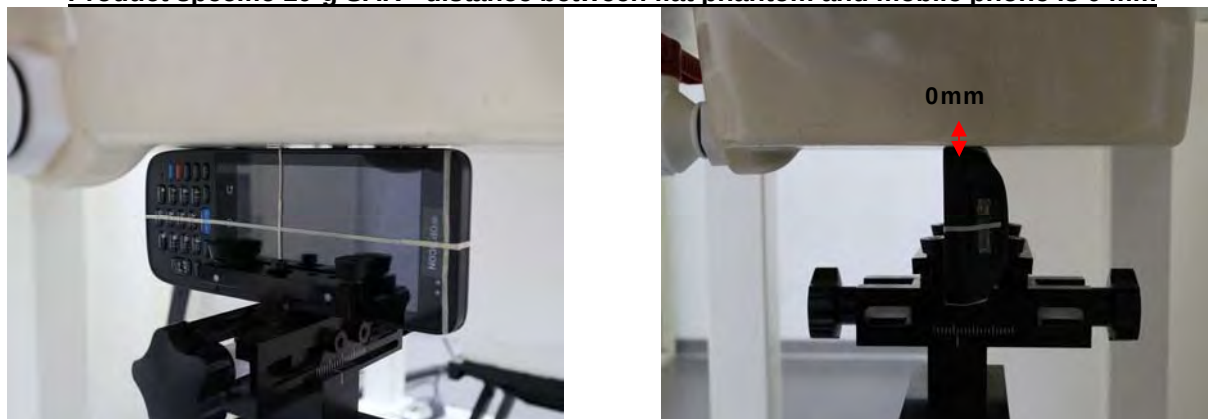
Fig.12 EUT Left side to flat phantom
