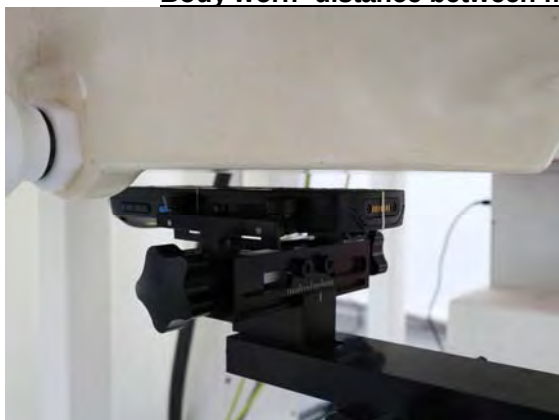
Fig.7 EUT Front side to flat phantom
