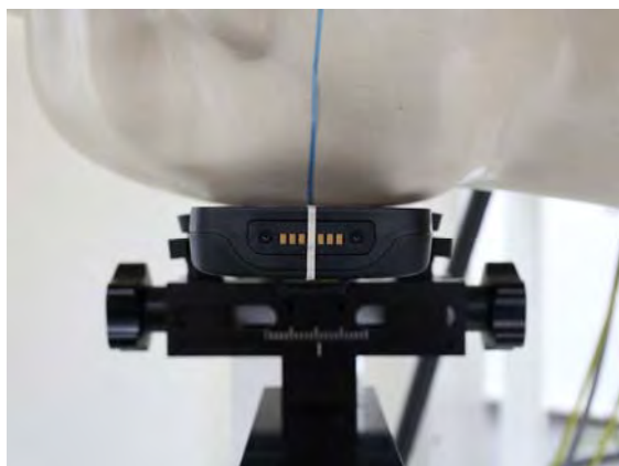
Fig.3 Right Head Section / Cheek-Touch Position
