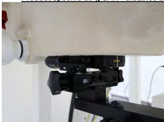
Fig.9 EUT Front side to flat phantom
