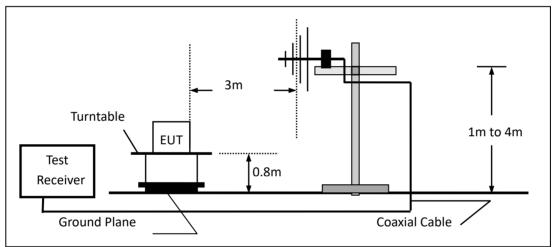
(c) For radiated emissions above 1000MHz
