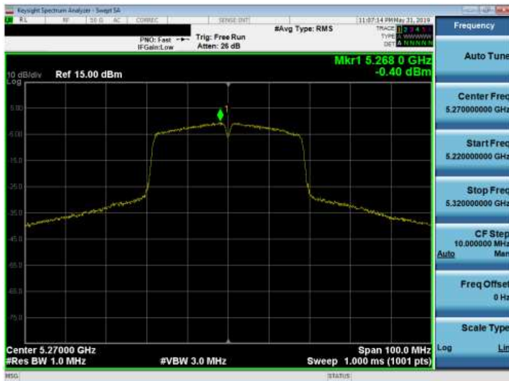
Plot 7-53. Power Spectral Density Plot (40MHz BW 802.11n (UNII Band 2A) – Ch. 54)
