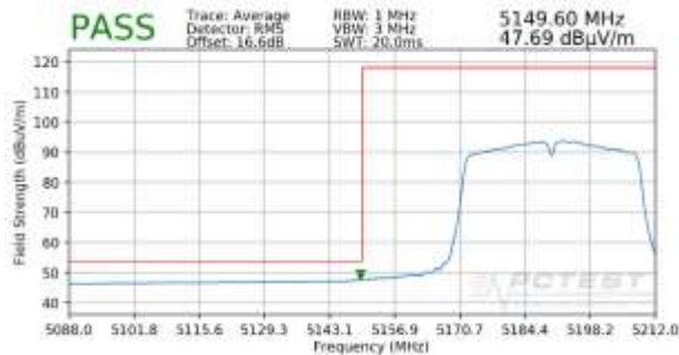
Plot 7-97. Radiated Lower Band Edge Plot (Average – UNII Band 1)
