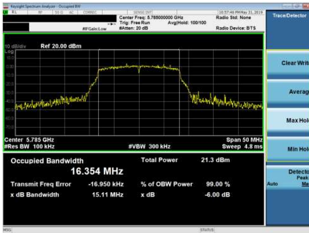
Plot 7-30. 6dB Bandwidth Plot (802.11a (UNII Band 3) – Ch. 157)
