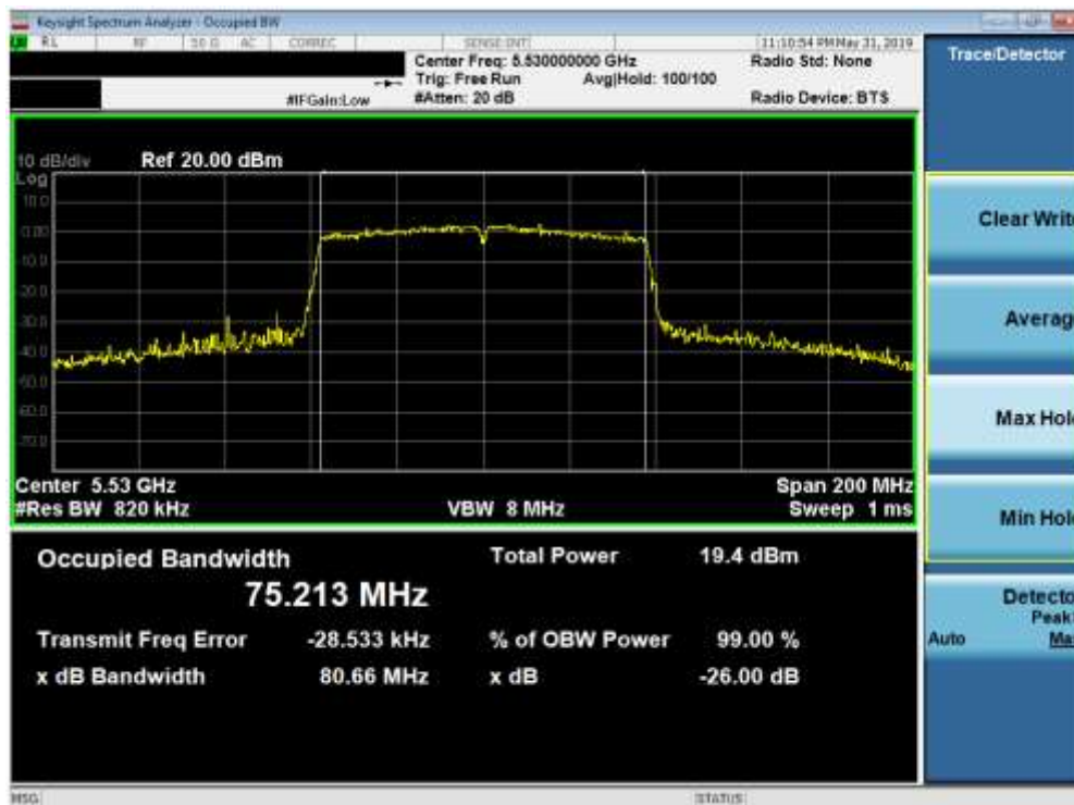
Plot 7-28. 26dB Bandwidth Plot (80MHz BW 802.11ac (UNII Band 2C) – Ch. 106)
