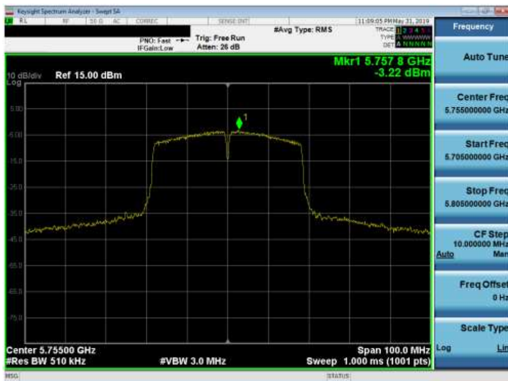
Plot 7-74. Power Spectral Density Plot (40MHz BW 802.11n (UNII Band 3) – Ch. 151)
