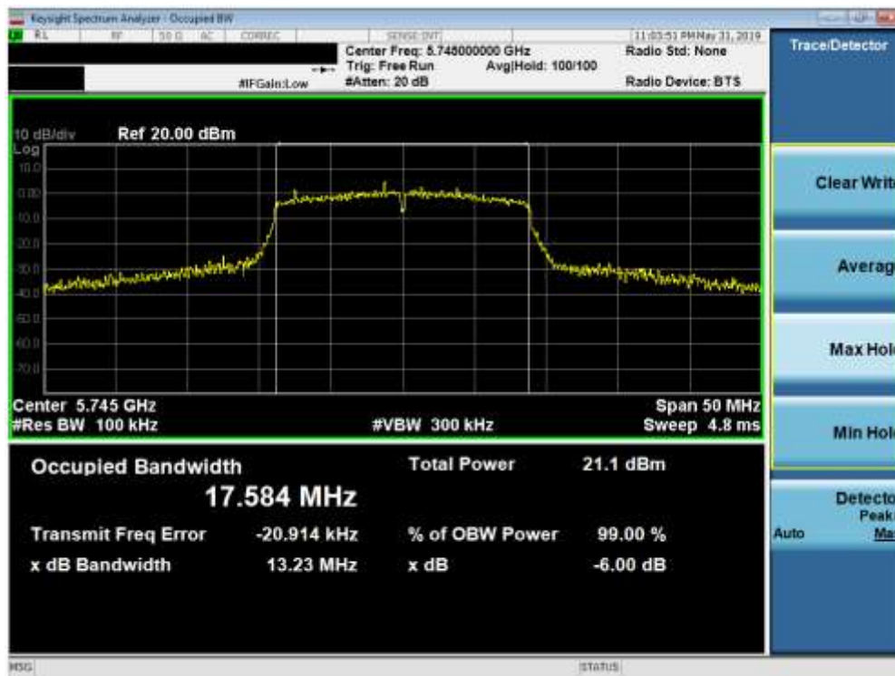
Plot 7-32. 6dB Bandwidth Plot (20MHz BW 802.11n (UNII Band 3) – Ch. 149)
