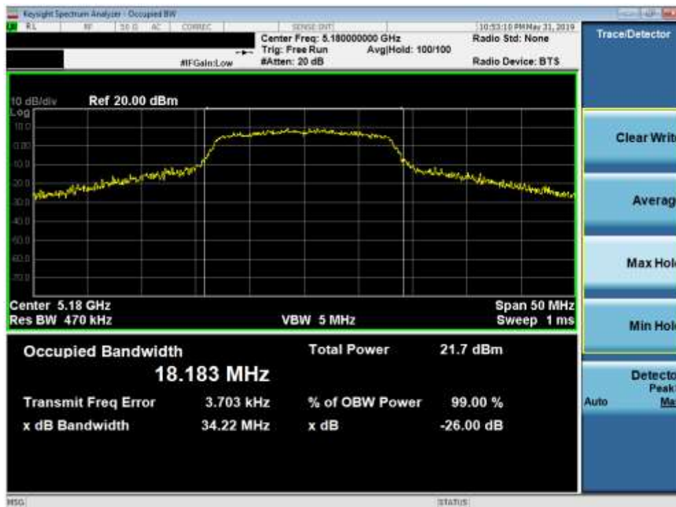
Plot 7-1. 26dB Bandwidth Plot (802.11a (UNII Band 1) – Ch. 36)
