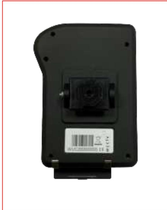
To mount the WCCTV Body Worn Camera, simply turn the body worn camera upside down and slide into the mount, then twist the body worn camera back into its upright position to secure.
