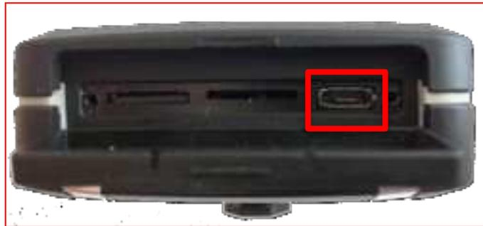
2. **Charging via the WCCTV Smart Hub:** Plug the WCCTV Smart Hub power adapter into the electrical supply and then insert the 2.1mm plug into the WCCTV Smart Hub. Place the WCCTV Body Worn Camera onto the WCCTV Smart Hub in one of the charging pockets provided.
