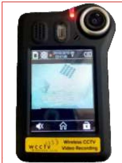
Whilst the WCCTV Body Worn Camera is recording, you can take a still image by tapping the screen, the unit will make a higher pitched beep to indicate the image has been taken.
