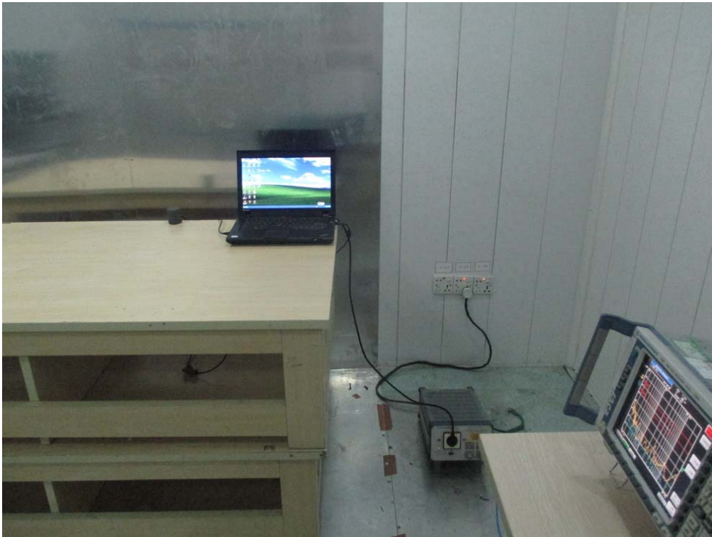
FCC RADIATED EMISSION TEST SETUP
