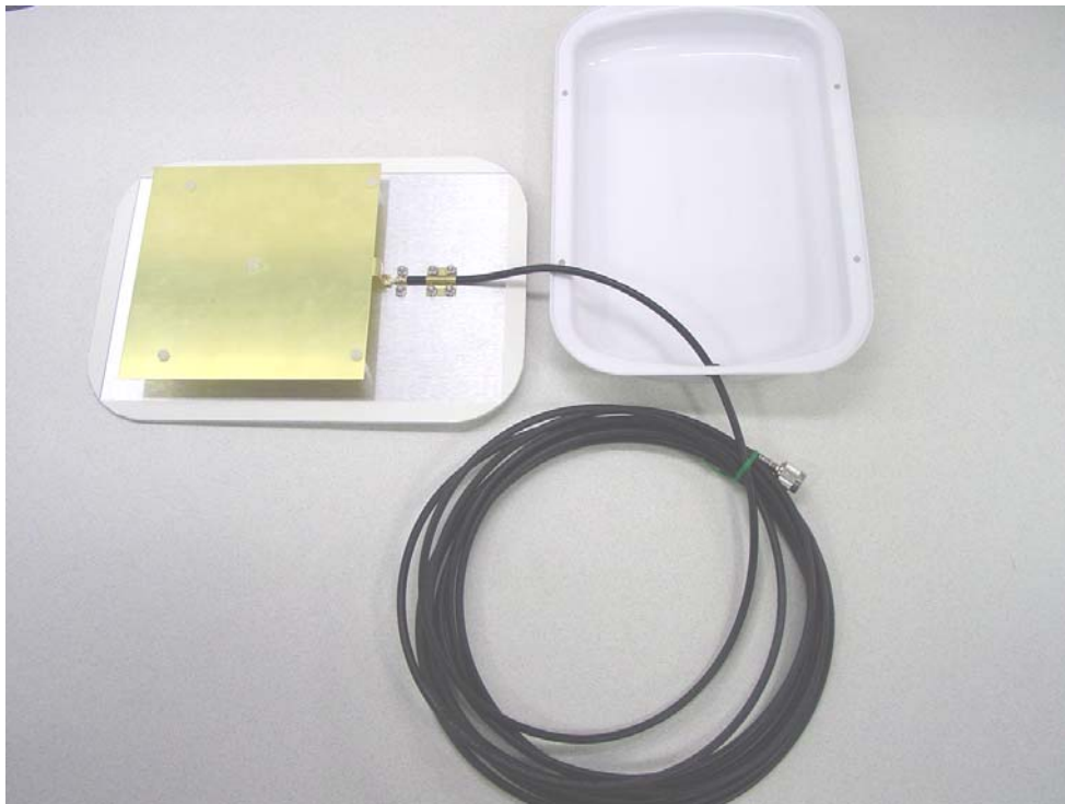
Linear Antenna Internal View
