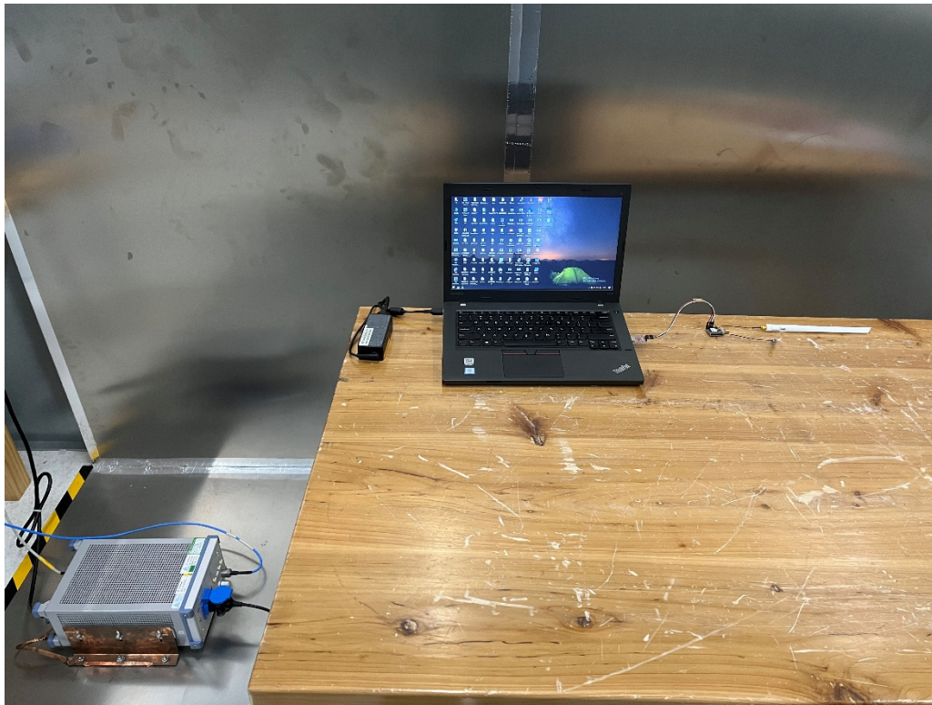
Photograph 3: Set-up for Conducted Emission on AC mains
