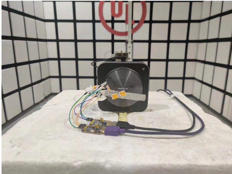
Radiated Disturbance Setup (Above 1 GHz – Z axis)
