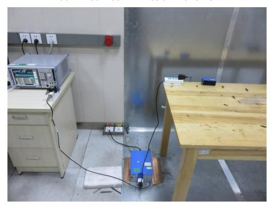
FCC RADIATED EMISSION TEST SETUP
