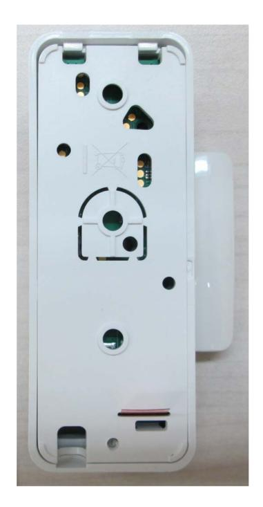
Photograph No.2 MC-309 PG2 magnetic contact rear side view
