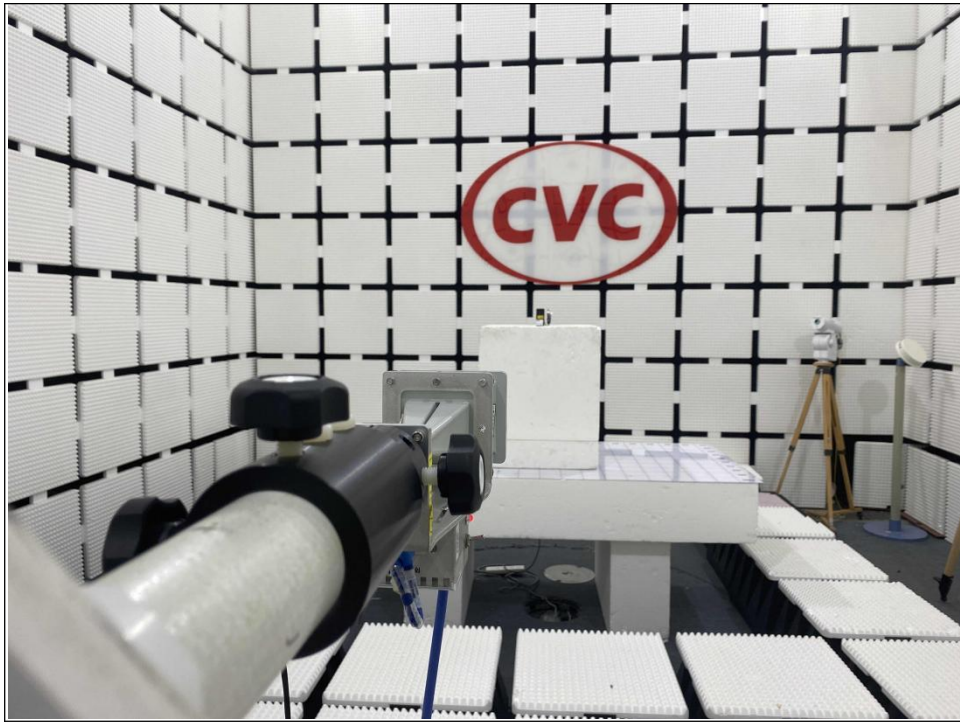
RADIATED EMISSION TEST (18GHz ~ 40GHz)
