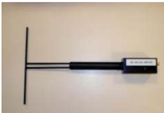
Figure 1 – MVG COMOSAR Validation Dipole
