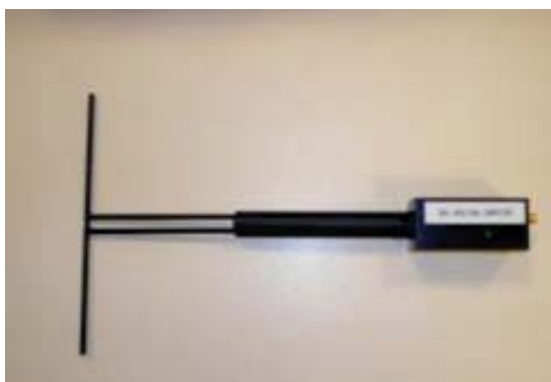
Figure 1 – MVG COMOSAR Validation Dipole
