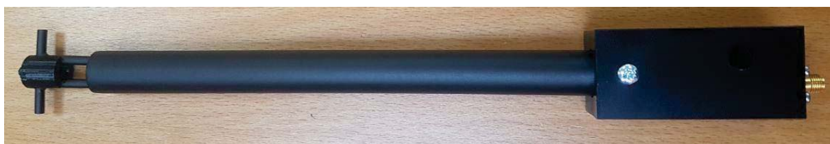
Figure 1 – MVG COMOSAR Validation Dipole
