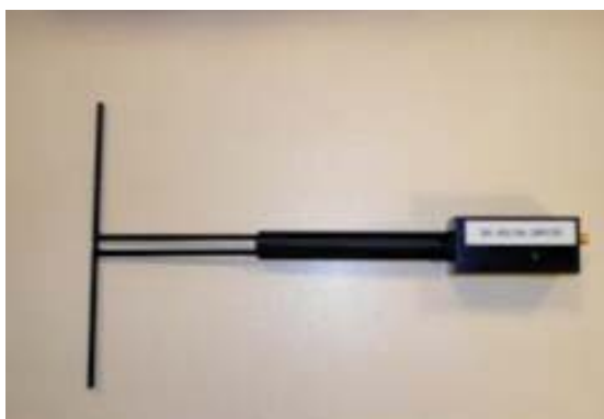
Figure 1 – MVG COMOSAR Validation Dipole
