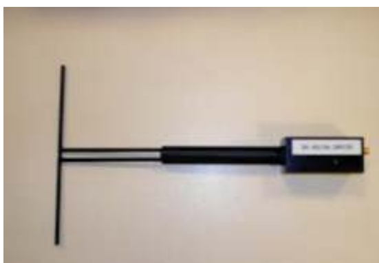
Figure 1 – MVG COMOSAR Validation Dipole
