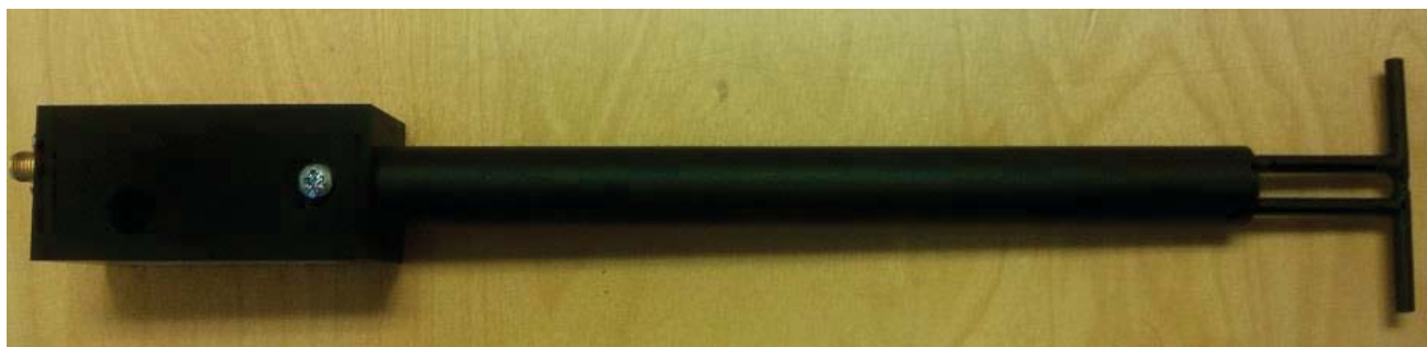
Figure 1 – MVG COMOSAR Validation Dipole
