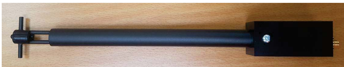
Figure 1 – MVG COMOSAR Validation Dipole
