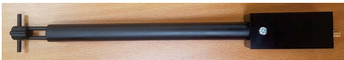
Figure 1 – MVG COMOSAR Validation Dipole
