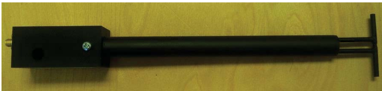
Figure 1 – MVG COMOSAR Validation Dipole
