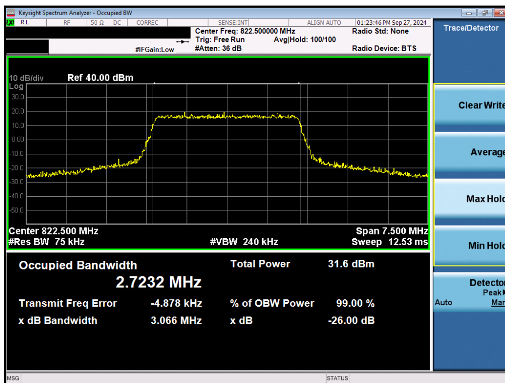
Plot 7-28. Occupied Bandwidth Plot (LTE Band 26 - 3MHz QPSK High Channel - Full RB)
