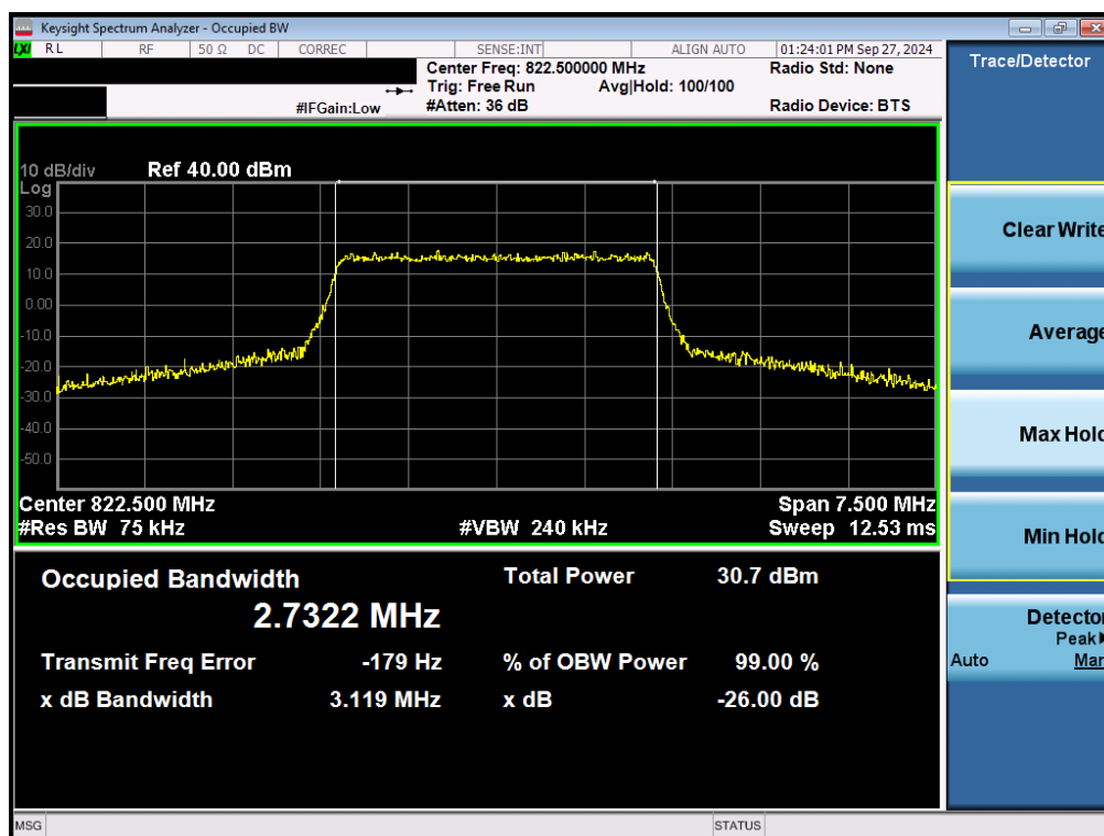
Plot 7-30. Occupied Bandwidth Plot (LTE Band 26 - 3MHz 16-QAM High Channel - Full RB)
