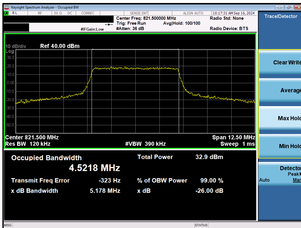
Plot 7-6. Occupied Bandwidth Plot (LTE Band 26 - 5MHz QPSK High Channel - Full RB)
