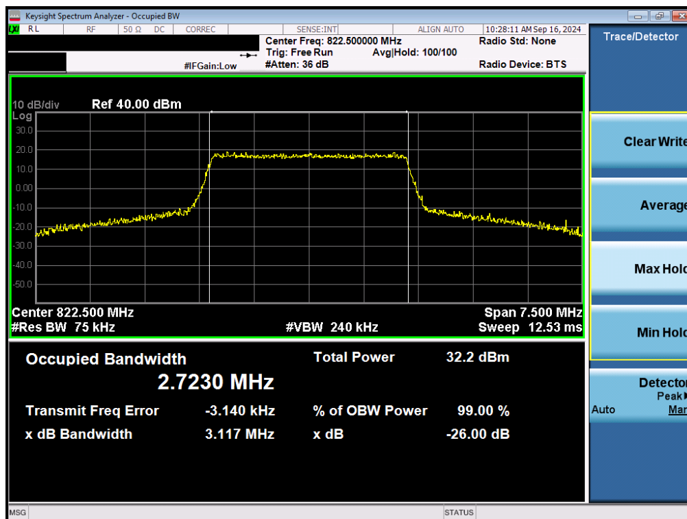
Plot 7-12. Occupied Bandwidth Plot (LTE Band 26 - 3MHz 16-QAM High Channel - Full RB)
