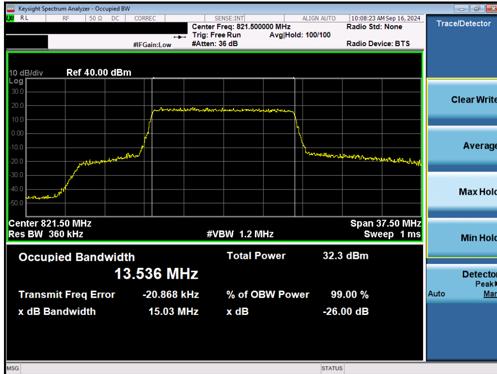
Plot 7-2. Occupied Bandwidth Plot (LTE Band 26 - 15MHz 16-QAM - Full RB)
