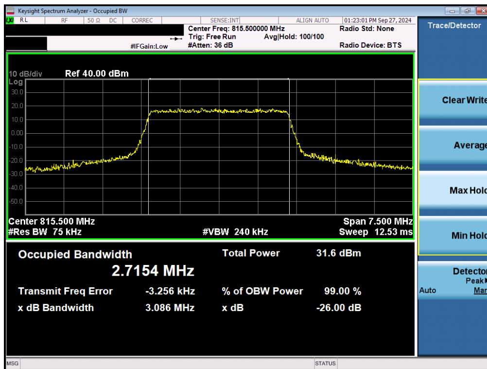
Plot 7-27. Occupied Bandwidth Plot (LTE Band 26 - 3MHz QPSK Low Channel- Full RB)
