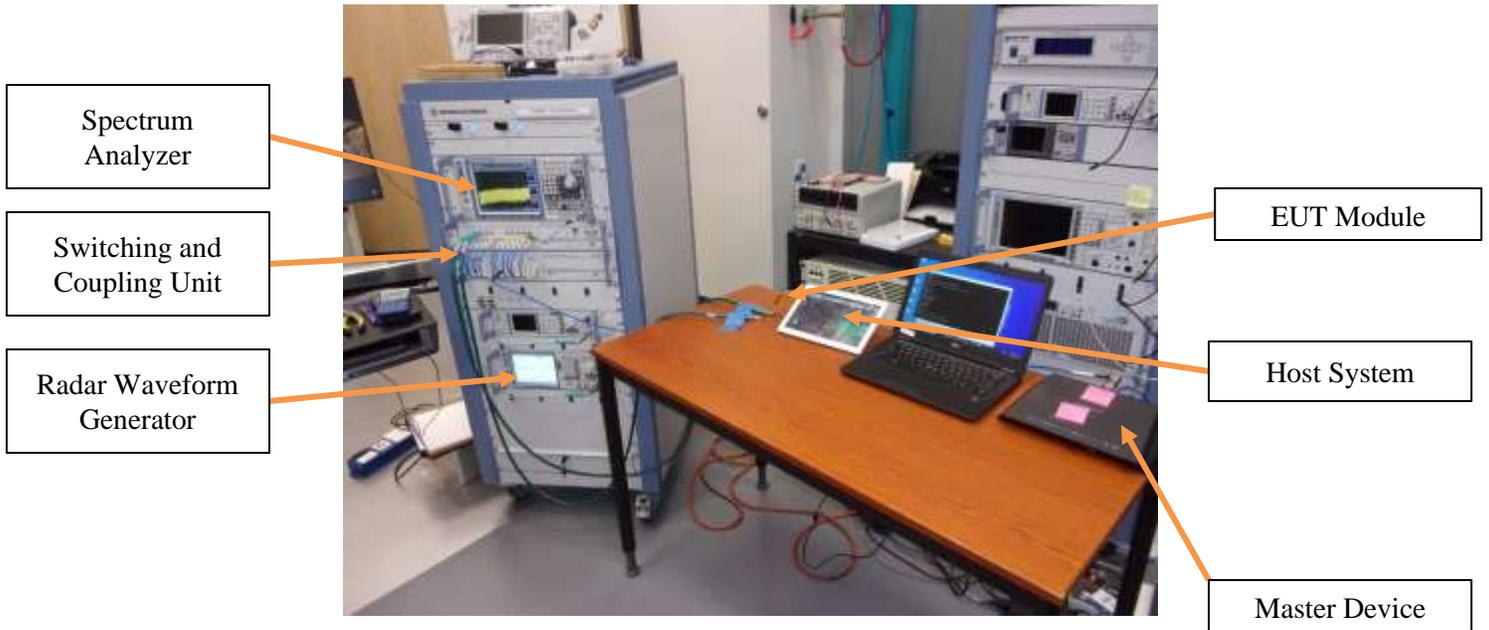
**Photograph 1: DFS Test Setup**
