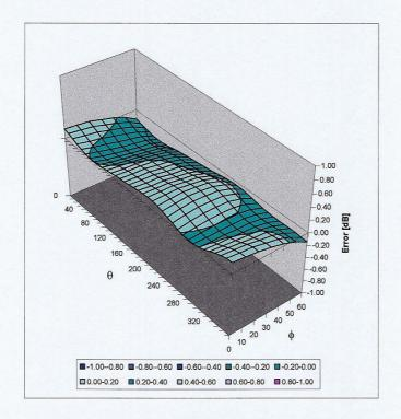
Spherical Isotropy Error < ± 0.4 dB
