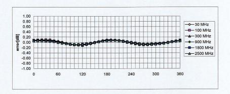
Axial Isotropy Error  $< \pm 0.2 \text{ dB}$
