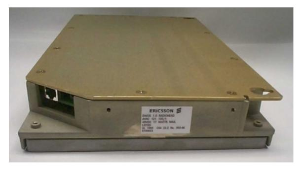
Front of Radio Head with TRX 3 antenna connector location, and RF shielded cover:
