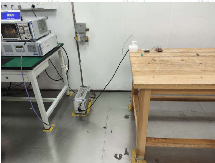
Conducted Emissions Test Setup
