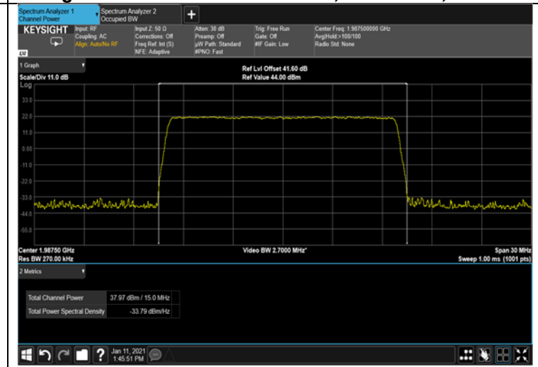
Figure 62: 256QAM 15MHz B.W.; 1987.5MHz, 30kHz
