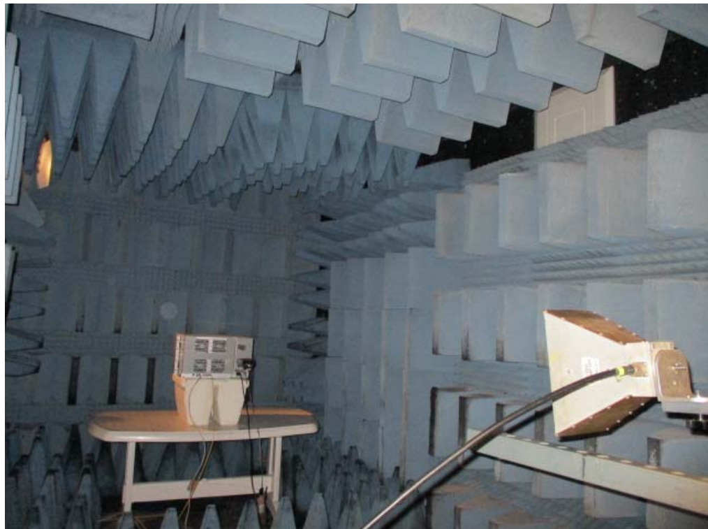
Figure 6. Radiated Emission Test 200 - 1000MHz
