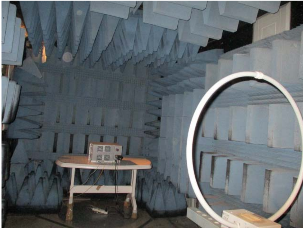
Figure 4. Radiated Emission Test 9kHz - 30MHz
