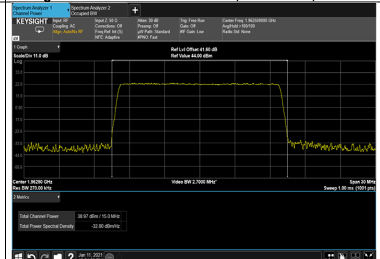
Figure 60: 256QAM 15MHz B.W.; 1962.5MHz, 30kHz
