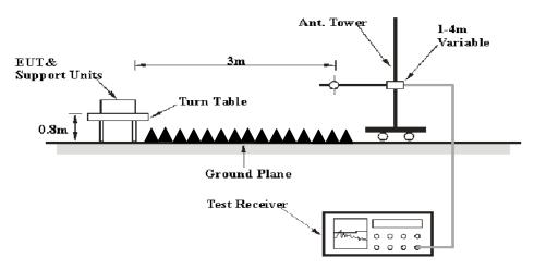
The radiated emission tests were performed in the 3 meters test site, using the setup accordance with the ANSI C63.4-2009. The specification used was the FCC 15.209, and FCC 15.247 limits.
