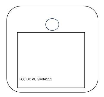
The label is located inside the battery compartment of the device.
