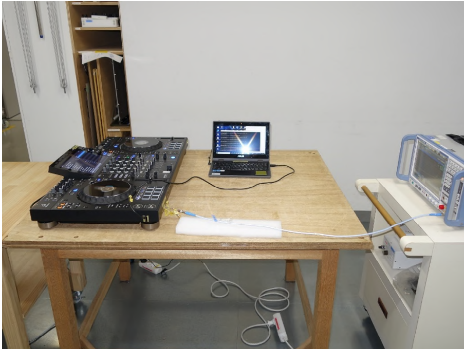
Photograph 1: Set-up for Antenna Port Conducted Emission of Transmitter
