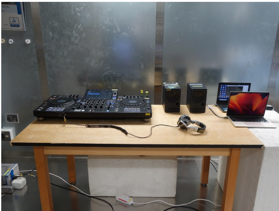
Photograph 8: Set-up for AC Power Line Conducted Emission, Front View
